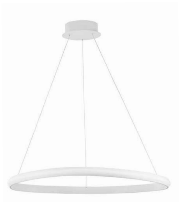
ARIES - 9357062 Dimmable Sandy White Aluminium & Acrylic LED 32 Watt 230 Volt 1770Lm 3000K IP20 D: 74 H: 120 cm
